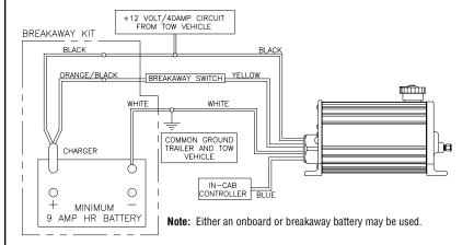
It is critical that the BLACK power lead and WHITE ground lead from the tow vehicle to the input of the actuator are sized and properly terminated (i.e. dedicated 25-40\* amp circuit on the tow vehicle – 12 gauge wire minimum). 10-gauge wire is recommended to optimize performance. Consult the SAE wiring guidelines for proper trailer electrical harness design.
