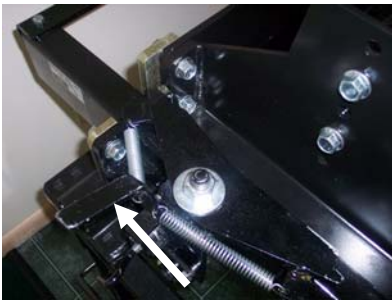
Figure 6.8 Retaining Pin location
