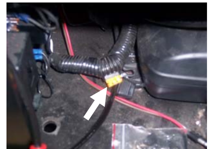
Figure 8.7 Wire loom fuse location
