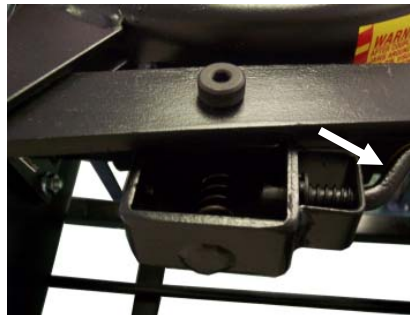
Figure 5.6 Retainer Pin view at Eight o'clock
