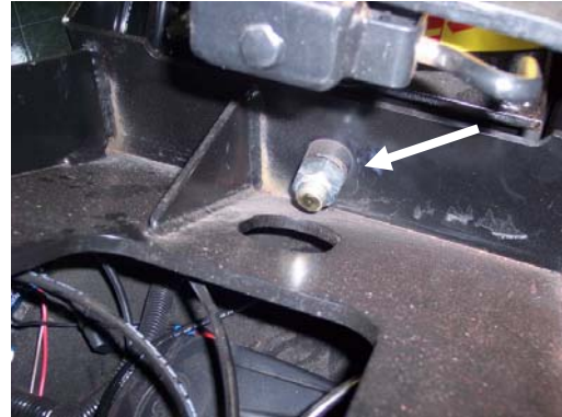
Figure 7.2 Check pivot bolt wear (PN 44031)
