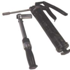
Figure 3.5 Torque wrench with \frac{3}{4} " socket & grease gun (PN N/A)
