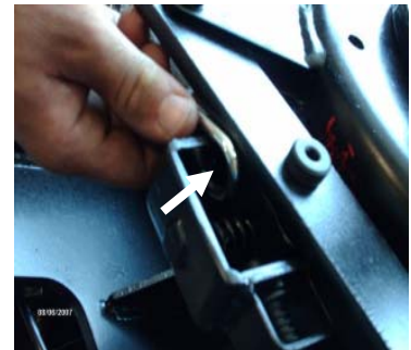
Figure 5.7 Padlock into Eight o'clock position
