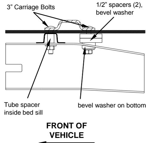
4. For the Row 4 passenger side attachment, stack two 1/2" spacers and a bevel washer, provided in the 58309 kit, to fill the gap between the bed and the frame. Use another bevel washer, conical toothed washer, and hex nut to fasten the 3" carriage bolt in place. See above drawing.
