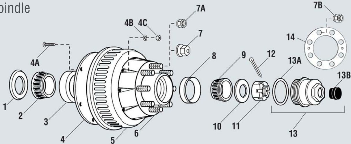
Electric or Hydraulic Hub and Drum Assembly
